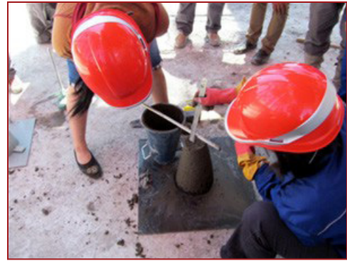
Technicians perform a slump test at the Premium Concrete batch plant.
