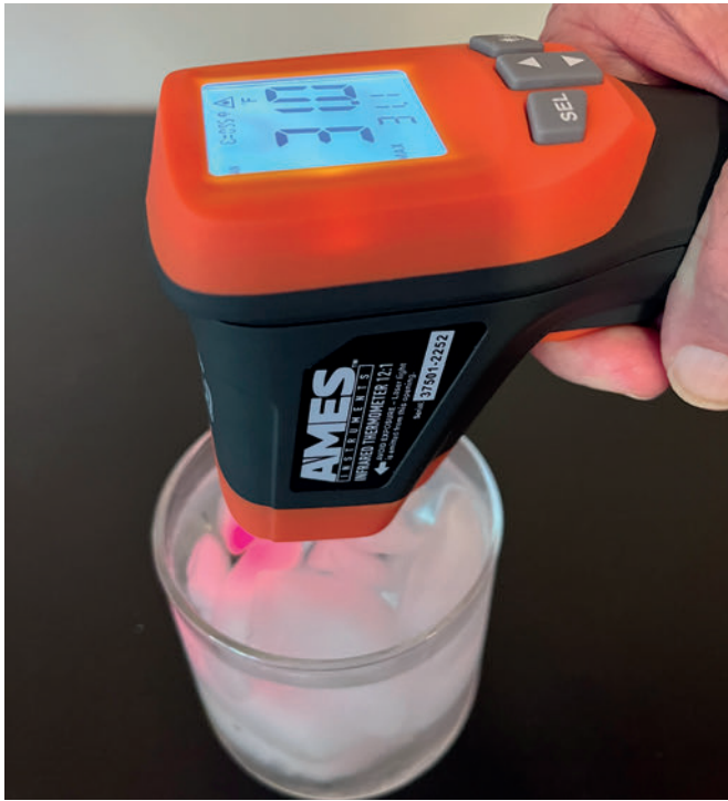
Performing the ice cube test: The IR thermometer is providing accurate readings if the indicated temperature is 32 F (0 °C) ±4 F (2 °C).
