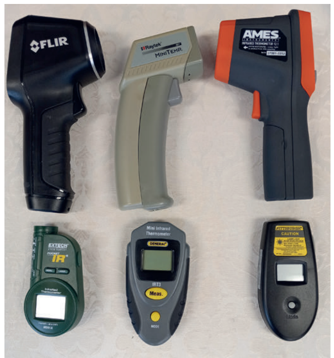
IR thermometers: Top row is the pistol type, bottom row is the pocket type.
