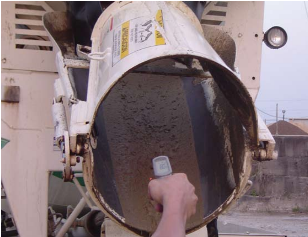
Fig. 1: Taking temperature measurements with an infrared thermometer is as easy as pointing at the object and pulling the trigger
